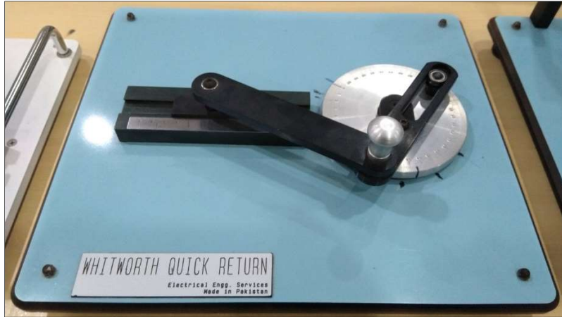
Figure 12: WhitWorth Quick Return Mechanism
