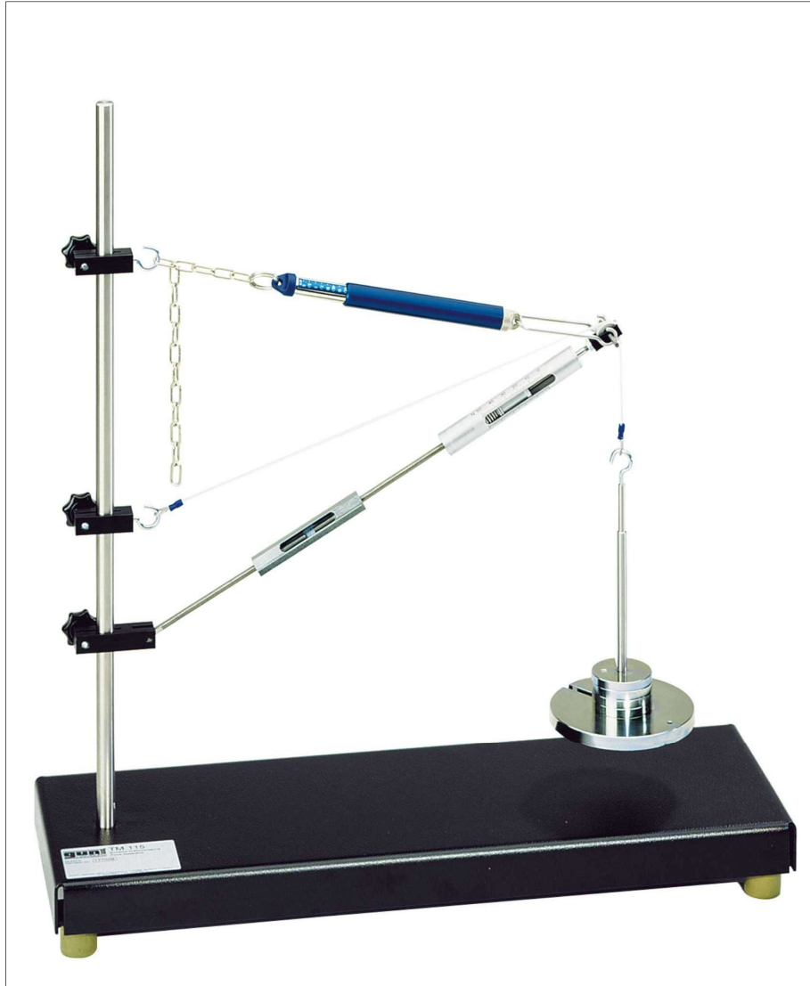
Figure 9: Forces on Crane Jig
