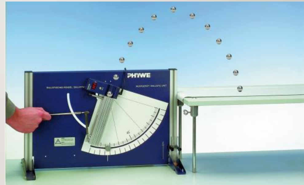
Experimental set-up for measuring the maximum range of a projectile with additional equipment to measure the initial velocity.
