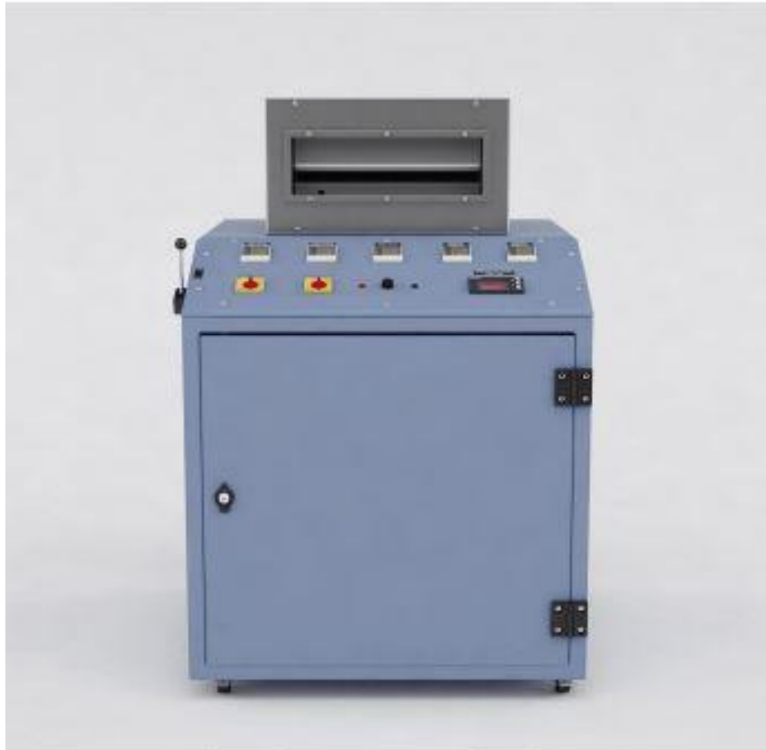
Figure 19: Conductivity unit for different building materials
