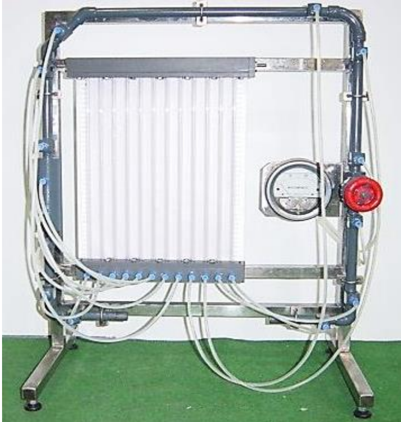
Figure 9: Energy Losses in Bends & Pipe fittings
